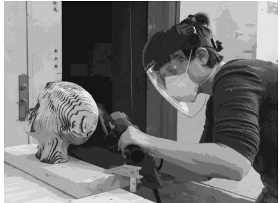
Using an angle grinder to sculpt stacked slices of laser cut plywood.
