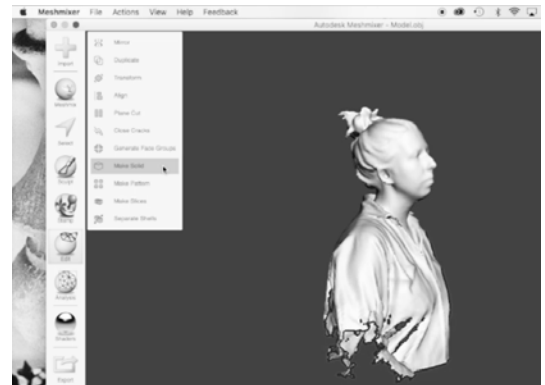
Raw scan getting turned into a solid model.
