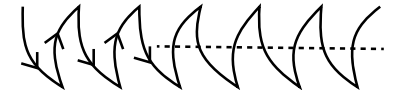
Ideal movement of welding gun along the seam of two pieces of metal. Imagine sewing them together.
